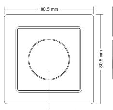
Click the rotary knob to switch ON/OFF paired Zigbee light devices
