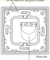
Battery: CR2450 Before the first use, please open the battery cover and remove the protective film
