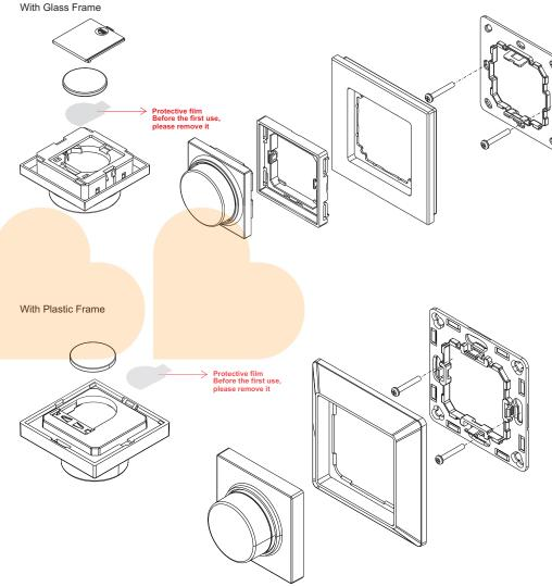
The key part of this controller is a universal, extremely rotary standard switch element that can be integrated in numerous frames by different manufactures as below list:
