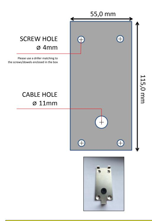
Please make sure when printing that the mounting plate dimension (width, height) fits to the actual print size. You can also use the original metal mounting plate as drilling template.
