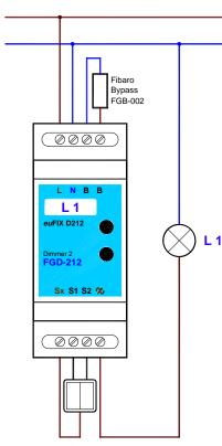
The descriptions of the screw terminals are printed on the adapter label. The sinusoid symbol with the arrow indicates the dimmer output, the letters "B" indicate contacts where the optional Fibaro Bypass FGB-002 can be connected.
