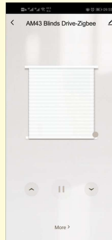
7. this page can operate the motor going UP, STOP, DOWN; click 'More' to get into multiple functions setting page
