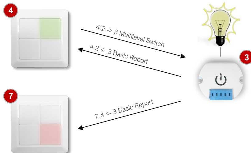
Figure 7: Multi-way switching with two MATRIX devices and a dimmer
