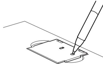
The red LED next to the learn in button will flash briefly then light up for approximately five seconds to show that it is ready to receive the "learn in" signal. During the next 5 seconds you will need to briefly press the test button on Alarm 1 to wirelessly interlink the two alarms.
