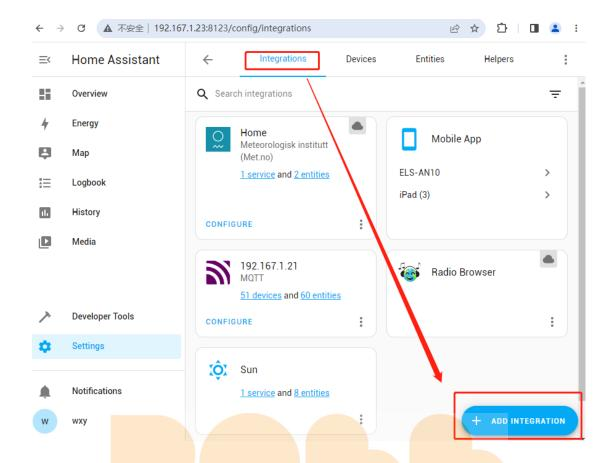
Step 3: In the pop-up dialog box, enter MQTT in the Search for a brand name input box, then select MQTT, as shown below:
