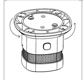
Turn right to dismantle the mounting base of the device
