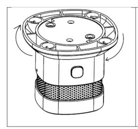
Turn left to install the mounting base of the device
