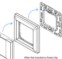
the frame and control part to the bracket in sequence
