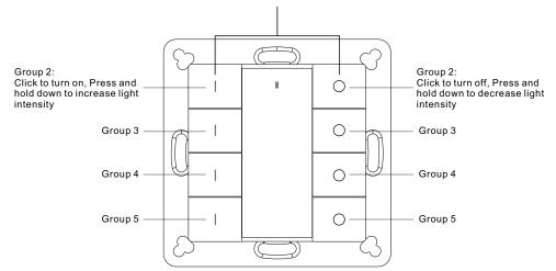
• Short press or press and hold down any button to send scene activation command to association group 1 using Command Class "Central Scene Notification V3".
