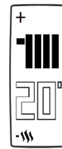
Radiator logo: a Valve located in a different room than the Thermostat requires heating
