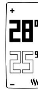
Flame logo: the Thermostat switches the heating on
