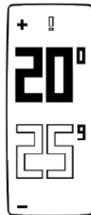
Exclamation mark: Relay not detected (loss of radio synchronization between Thermostat and Relay)
